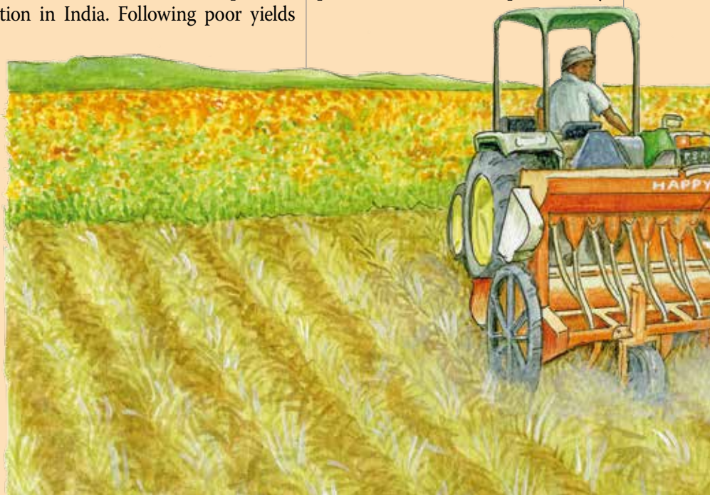
Zero-tillage in action: the 'Happy Seeder' drills wheat seeds through heavy loads of rice crop residues
