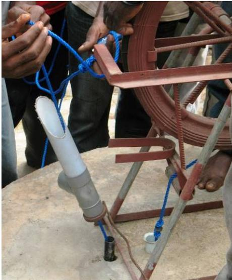
1) Tread the rope with piston going out of the PVC trough the T pipe
